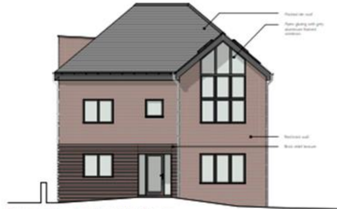
Proposed House - Front (South West) Elevation
