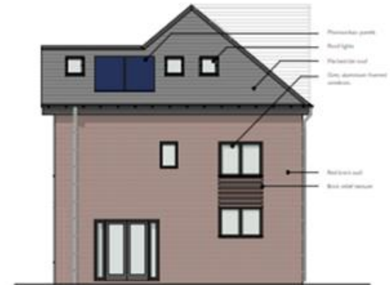
Proposed House - Side (South East) Elevation
